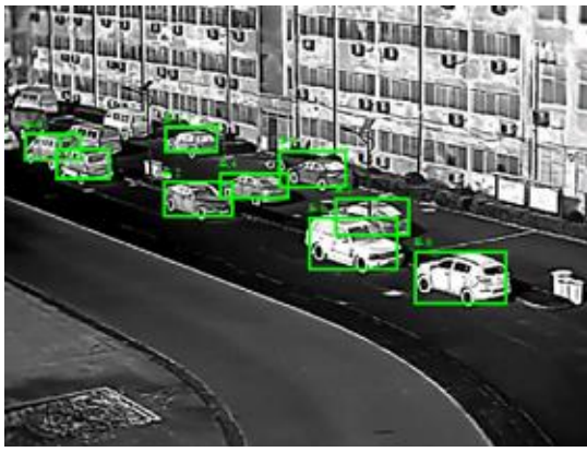
Dual band imaging and target recognition using thermal infrared and visible light
